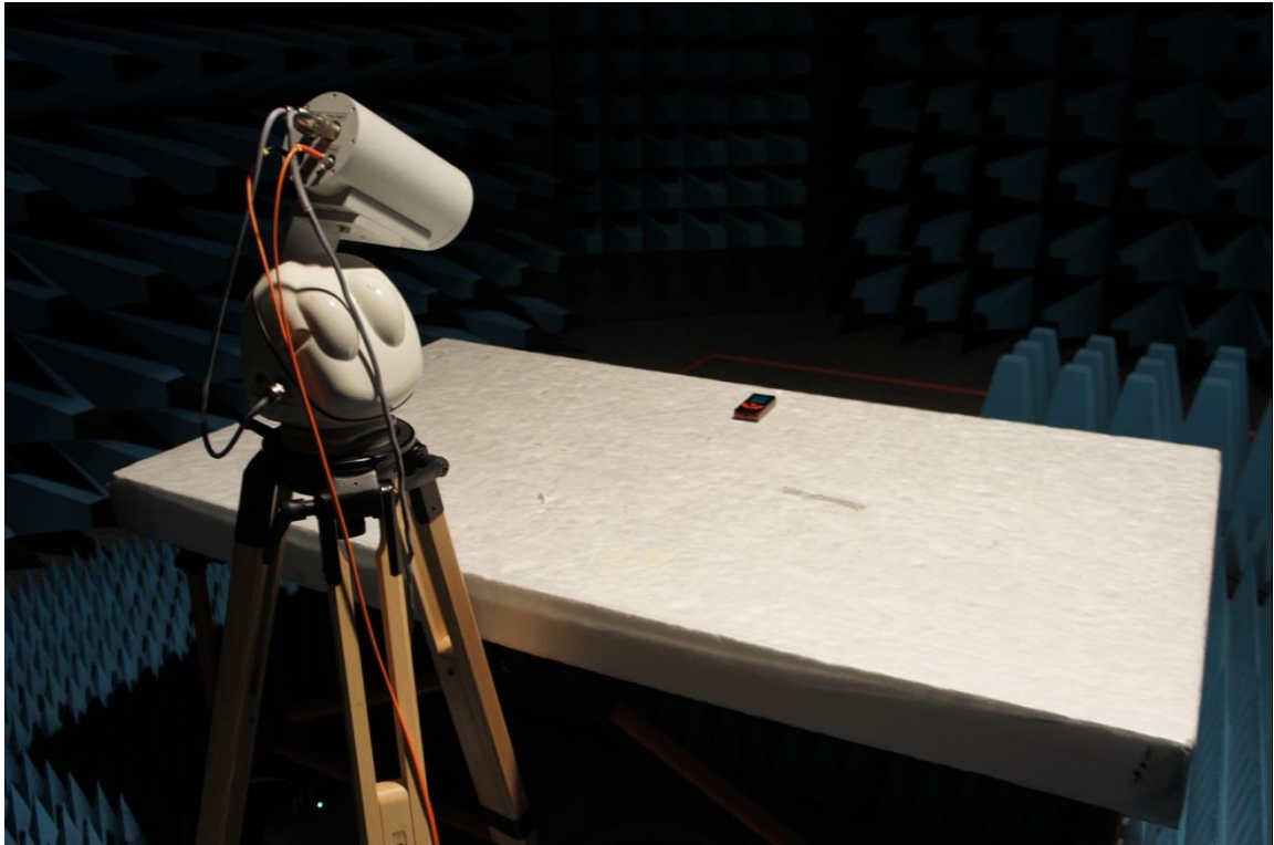
Picture 5: Test setup radiated immunity test
